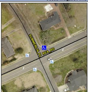
SUMMERLIN PL Street 1 Name Stop Condition-Street 2 StopSign **REA RD** Street 2 Name Stop Condition-Street 1 None Possible Solutions: Remove & Replace Curb Ramp With Two New Directional Ramps or Equivalent. Surveyor Notes: N/A PROW/ADA: R304.5.1, R304.5.3
