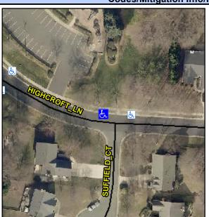
**HIGHCROFT LN** Street 1 Name Stop Condition-Street 1 None N/A Street 2 Name Stop Condition-Street 2 N/A Possible Solutions: Remove & Replace Curb Ramp With Two New Directional Ramps or Equivalent. Surveyor Notes: N/A PROW/ADA: Not Found, R304.5.3
