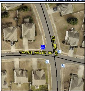
**CACTUS VALLEY RD** Street 1 Name Stop Condition-Street 2 None **DEL RIO RD** Street 2 Name Stop Condition-Street 1 StopSign Possible Solutions: Remove & Replace Curb Ramp With Two New Directional Ramps or Equivalent. Surveyor Notes: N/A PROW/ADA: Not Found, R304.5.1, R304.5.3
