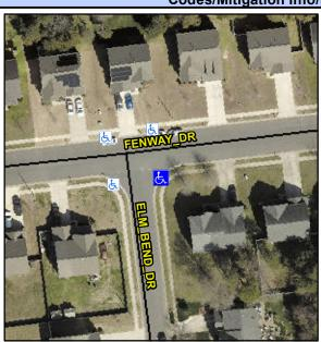
**FENWAY DR** Street 1 Name Stop Condition-Street 2 None **ELM BEND DR** Street 2 Name Stop Condition-Street 1 StopSign Possible Solutions: N/A Remove & Replace Curb Ramp With Two New Directional Ramps or Yes Equivalent. N/A N/A N/A N/A Surveyor Notes: N/A N/A N/A N/A N/A PROW/ADA: N/A R304.2.2, R304.5.3 N/A N/A N/A N/A
