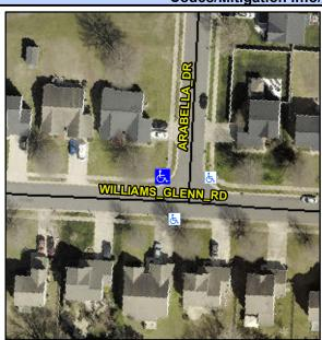
WILLIAMS GLENN RD Street 1 Name Stop Condition-Street 2 None Street 2 Name **ARABELLA DR** Stop Condition-Street 1 StopSign Possible Solutions: **Remove & Replace Curb Ramp With Two New Directional Ramps or** Equivalent. Surveyor Notes: N/A PROW/ADA: R304.5.3
