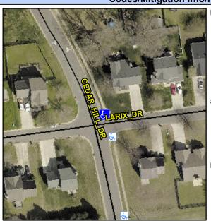
Possible Solutions: Remove & Replace Curb Ramp With Two New Directional Ramps or Equivalent.
