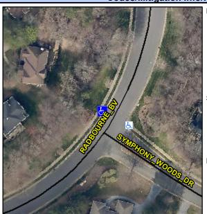
**RADBOURNE BV** Street 1 Name Stop Condition-Street 2 None N/A Street 2 Name Stop Condition-Street 1 N/A Possible Solutions: Remove & Replace Entire Ramp. Surveyor Notes: N/A PROW/ADA: R304.2.2
