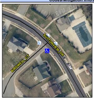
Street 1 Name Stop Condition-Street 2 Street 2 Name Stop Condition-Street 1 **SUTTONVIEW DR** None **BIRDWELL CT** StopSign Possible Solutions: Remove & Replace Curb Ramp With **Two New Directional Ramps or** Equivalent. Surveyor Notes: N/A PROW/ADA: Not Found, R304.5.1
