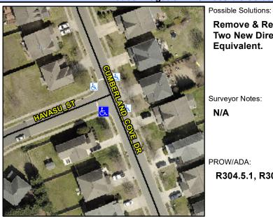
**CUMBERLAND COVE DR** Street 1 Name Stop Condition-Street 2 StopSign Street 2 Name **HAVASU ST** Stop Condition-Street 1 StopSign **Remove & Replace Curb Ramp With Two New Directional Ramps or** Equivalent.
