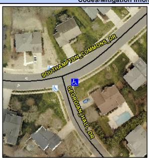
SOUTHAMPTON COMMONS DR Street 1 Name Stop Condition-Street 2 None **GEORGIAN HALL DR** Street 2 Name Stop Condition-Street 1 StopSign Possible Solutions: Remove & Replace Curb Ramp With Two New Directional Ramps or Equivalent. Surveyor Notes: N/A
