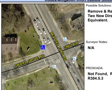
**BEATTIES FORD RD** Street 1 Name Stop Condition-Street 2 Signal Street 2 Name **CINDY LN** Stop Condition-Street 1 Signal Remove & Replace Curb Ramp With Two New Directional Ramps or Equivalent.
