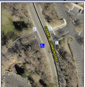
**CARMEL COMMONS BV** Street 1 Name Stop Condition-Street 2 None **ENTRANCE** Street 2 Name Stop Condition-Street 1 StopSign Possible Solutions: Remove & Replace Curb Ramp With Two New Directional Ramps or Equivalent. Surveyor Notes:
