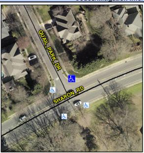
Street 1 Name Stop Condition-Street 1 Street 2 Name Stop Condition-Street 2 **QUAIL PARK DR** StopSign **SHARON RD** None Possible Solutions: Remove & Replace Curb Ramp With Two New Directional Ramps or Equivalent. Surveyor Notes: N/A
