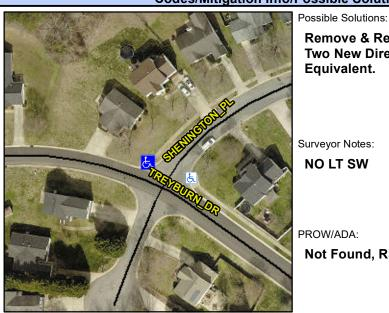
SHENINGTON PL Street 1 Name Stop Condition-Street 1 StopSign Street 2 Name N/A Stop Condition-Street 2 N/A Remove & Replace Curb Ramp With **Two New Directional Ramps or** Equivalent.
