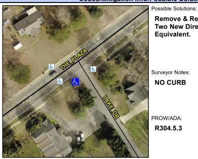
LAKE DR Street 1 Name Stop Condition-Street 1 StopSign Street 2 Name N/A Stop Condition-Street 2 N/A **Remove & Replace Curb Ramp With Two New Directional Ramps or** Equivalent.
