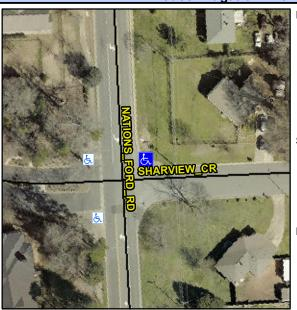
Street 1 Name Stop Condition-Street 2 Street 2 Name Stop Condition-Street 1 NATIONS FORD RD None **SHARVIEW CR** StopSign Possible Solutions: Remove & Replace Curb Ramp With Two New Directional Ramps or Equivalent. Surveyor Notes: N/A PROW/ADA: Not Found, R304.2.2, R304.5.3, R302.7
