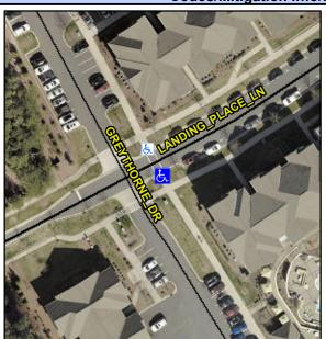
LANDING PLACE LN Street 1 Name Stop Condition-Street 1 None N/A Street 2 Name Stop Condition-Street 2 N/A Possible Solutions: Remove & Replace Curb Ramp With Two New Directional Ramps or Equivalent. Surveyor Notes: N/A
