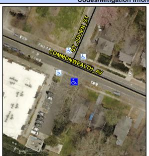
ST JULIEN ST Street 1 Name Stop Condition-Street 2 None Street 2 Name N/A Stop Condition-Street 1 N/A Possible Solutions: Remove & Replace Entire Ramp. Remove & Replace Gutter. Surveyor Notes: N/A PROW/ADA: Not Found, R304.2.1, R304.2.2-Perp, R304.3.2-Para, R305.1.4, R305.2, R304.5.4, R304.5.3
