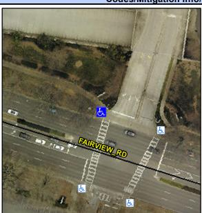
**FAIRVIEW RD** Street 1 Name Stop Condition-Street 2 Signal **ENTRANCE** Street 2 Name Stop Condition-Street 1 Signal Possible Solutions: Remove & Replace Curb Ramp With Two New Directional Ramps or Equivalent. Surveyor Notes: N/A PROW/ADA: R304.5.3
