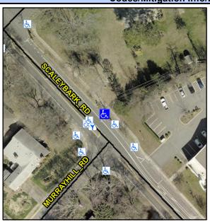
Street 1 Name None Stop Condition-Street 1 SCALEYBARK RD N/A Street 2 Name Stop Condition-Street 2 N/A Possible Solutions: Remove & Replace Entire Ramp. Surveyor Notes: N/A PROW/ADA: Not Found, R304.2.2, R304.3.2
