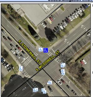
Street 1 Name Signal **S MCDOWELL ST** Stop Condition-Street 1 Street 2 Name N/A Stop Condition-Street 2 N/A Possible Solutions: Remove & Replace Entire Ramp. Remove & Replace Gutter. Surveyor Notes: **RT RP < 5%** PROW/ADA: Not Found, R304.5.3, R304.2.1, R304.2.2-Perp, R304.3.2-Para
