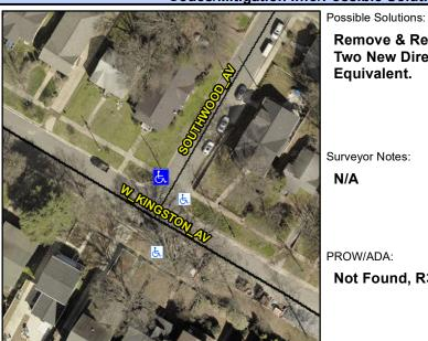
**SOUTHWOOD AV** Street 1 Name StopSign Stop Condition-Street 1 Street 2 Name N/A Stop Condition-Street 2 N/A Remove & Replace Curb Ramp With **Two New Directional Ramps or** Equivalent.
