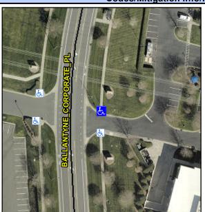
Street 1 Name **ENTRANCE** Stop Condition-Street 1 StopSign Street 2 Name N/A Stop Condition-Street 2 N/A Possible Solutions: **Remove & Replace Curb Ramp With** Two New Directional Ramps or Equivalent. Surveyor Notes: N/A PROW/ADA: R304.5.3
