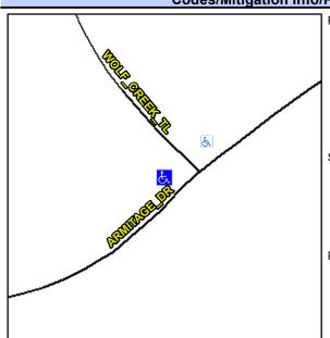
**WOLF CREEK TL** Street 1 Name Stop Condition-Street 1 StopSign Street 2 Name N/A Stop Condition-Street 2 N/A Possible Solutions: Remove & Replace Entire Ramp. Remove & Replace Gutter. Surveyor Notes: N/A PROW/ADA: Not Found, R304.2.2-Perp, R304.3.2-Para, R304.5.3, R304.5.2, R305.2, R302.7.2
