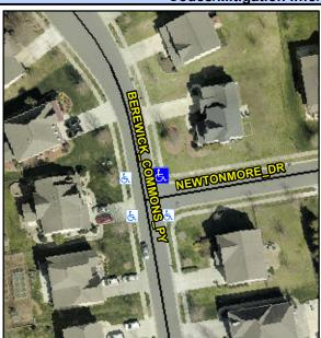
Street 1 Name **BEREWICK COMMONS PY** Stop Condition-Street 2 **NEWTONMORE DR** Street 2 Name Stop Condition-Street 1 StopSign Possible Solutions: Remove & Replace Curb Ramp With Two New Directional Ramps or Equivalent. Surveyor Notes: N/A PROW/ADA: R304.5.1, R304.5.3
