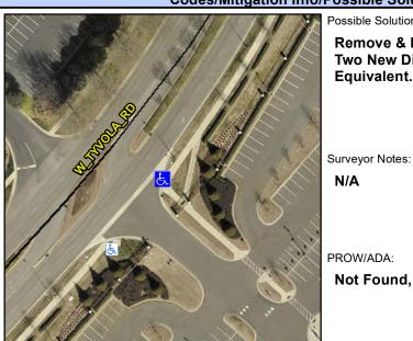
**ENTRANCE** Street 1 Name Stop Condition-Street 1 StopSign Street 2 Name N/A Stop Condition-Street 2 N/A Possible Solutions: Remove & Replace Curb Ramp With **Two New Directional Ramps or** Equivalent.
