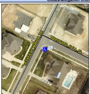
**DEERFIELD MANOR DR** Street 1 Name Stop Condition-Street 2 None Street 2 Name N/A Stop Condition-Street 1 N/A Possible Solutions: Remove & Replace Entire Ramp. Remove & Replace Gutter. Surveyor Notes: N/A PROW/ADA: Not Found, R305.2, R302.7.2, R304.5.4
