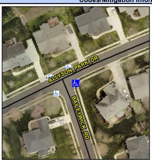
Street 1 Name Stop Condition-Street 2 Street 2 Name Stop Condition-Street 1 **ALLYSON PARK DR** None **BAILEYWICK RD** StopSign Possible Solutions: **Remove & Replace Curb Ramp With Two New Directional Ramps or** Equivalent. Surveyor Notes: N/A PROW/ADA: Not Found, R304.5.1, R304.5.3
