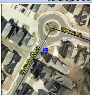
SAPPHIRE HILL LN Street 1 Name Stop Condition-Street 2 YieldSign Street 2 Name N/A Stop Condition-Street 1 N/A Possible Solutions: Remove & Replace Entire Ramp. Gutter Ponding Observed. Surveyor Notes: N/A PROW/ADA: R304.2.2-Perp, R304.3.2-Para, R304.5.3, R304.2.3, R302.7
