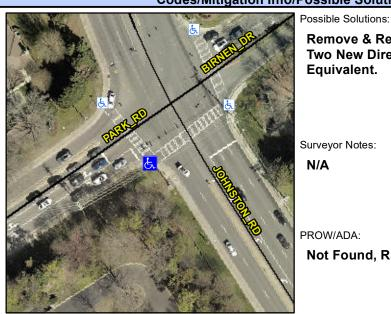
**JOHNSTON RD** Street 1 Name Stop Condition-Street 2 Signal Street 2 Name **PARK RD** Stop Condition-Street 1 Signal Remove & Replace Curb Ramp With Two New Directional Ramps or Equivalent.
