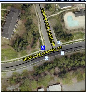
**ROZZELLES LANDING DR** Street 1 Name Stop Condition-Street 2 **CODDINGTON RIDGE DR** Street 2 Name Stop Condition-Street 1 StopSign Possible Solutions: Compliance Description Remove & Replace Curb Ramp With Two New Directional Ramps or Equivalent. Surveyor Notes: N/A PROW/ADA: Not Found, R304.5.1
