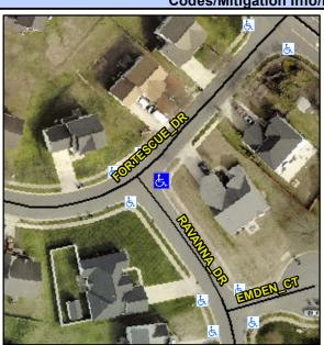
Street 1 Name Stop Condition-Street 2 Street 2 Name Stop Condition-Street 1 **FORTESCUE DR** None **RAVANNA DR** StopSign Possible Solutions: Remove & Replace Curb Ramp With Two New Directional Ramps or Equivalent. Surveyor Notes: N/A PROW/ADA: Not Found, R304.5.3
