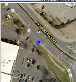
Street 1 Name Stop Condition-Street 2 Street 2 Name Stop Condition-Street 1 **SANDY PORTER RD** None **ENTRANCE** StopSign Possible Solutions: Remove & Replace Curb Ramp With **Two New Directional Ramps or** Equivalent. Surveyor Notes: N/A PROW/ADA: Not Found, R304.5.1, R304.2.2, R304.5.3
