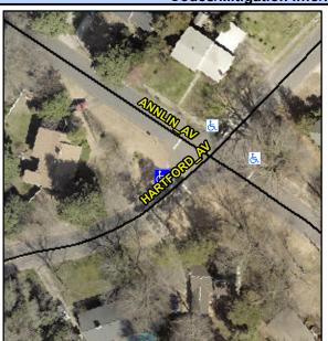
Street 1 Name Stop Condition-Street 2 Street 2 Name Stop Condition-Street 1 HARTFORD AV StopSign **ANNLIN AV** StopSign Possible Solutions: **Remove & Replace Curb Ramp With** Two New Directional Ramps or Equivalent.
