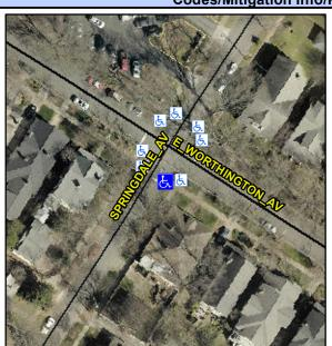
**SPRINGDALE AV** Street 1 Name Stop Condition-Street 2 StopSign Street 2 Name N/A Stop Condition-Street 1 N/A Possible Solutions: Remove & Replace Entire Ramp. Surveyor Notes: N/A PROW/ADA: Not Found, R304.2.2, R304.5.3
