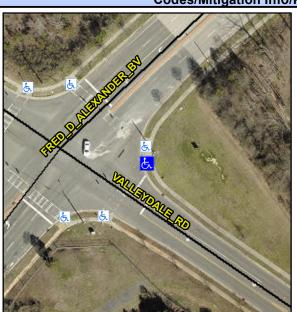
Street 1 Name Signal Stop Condition-Street 1 VALLEYDALE RD N/A Street 2 Name Stop Condition-Street 2 N/A Possible Solutions: Remove & Replace Entire Ramp. Remove & Replace Gutter. Surveyor Notes: GTR GAP 1.5", RP < 5% PROW/ADA Not Found, R305.1.4, R305.2, R304.5.4
