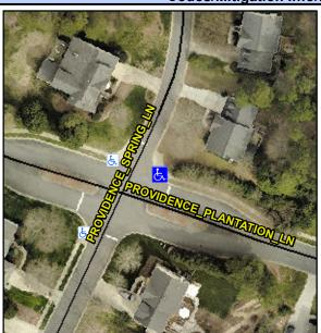
PROVIDENCE SPRING LN Street 1 Name Stop Condition-Street 2 StopSign Street 2 Name N/A Stop Condition-Street 1 N/A Possible Solutions: Remove & Replace Entire Ramp. Surveyor Notes: N/A PROW/ADA: Not Found, R304.5.3
