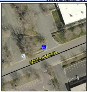
Street 1 Name Stop Condition-Street 2 Street 2 Name Stop Condition-Street 1 **CENTER PARK DR** None **ENTRANCE** None Possible Solutions: Remove & Replace Curb Ramp With **Two New Directional Ramps or** Equivalent. Surveyor Notes: N/A PROW/ADA: Not Found, R304.5.1, R304.2.2
