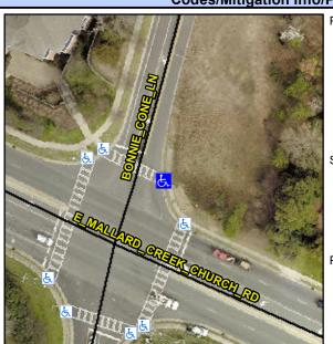
**BONNIE CONE LN** Street 1 Name Stop Condition-Street 2 Signal Street 2 Name N/A Stop Condition-Street 1 N/A Possible Solutions: Remove & Replace Entire Ramp. Surveyor Notes: N/A PROW/ADA: R304.5.1, R304.2.2
