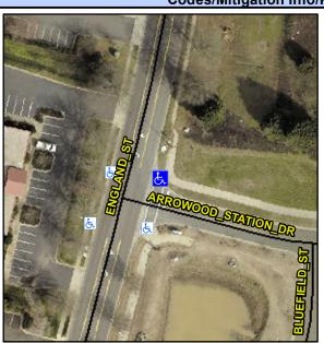
**ENGLAND ST** Street 1 Name Stop Condition-Street 2 None ARROWOOD STATION DR Street 2 Name Stop Condition-Street 1 StopSign Possible Solutions: Remove & Replace Curb Ramp With Two New Directional Ramps or Equivalent. Surveyor Notes: N/A PROW/ADA: Not Found, R304.2.2
