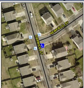
Street 1 Name Stop Condition-Street 2 Street 2 Name Stop Condition-Street 1 **NEWFIELD ST** StopSign **DARWICK ST** None Possible Solutions: Remove & Replace Curb Ramp With **Two New Directional Ramps or** Equivalent. Surveyor Notes: N/A PROW/ADA: Not Found, R304.5.1
