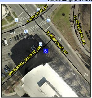
**E MOREHEAD ST** Street 1 Name Stop Condition-Street 1 None N/A Street 2 Name Stop Condition-Street 2 StopSign Possible Solutions: Remove & Replace Curb Ramp With Two New Directional Ramps or Equivalent. Surveyor Notes: N/A PROW/ADA: Not Found, R304.5.1
