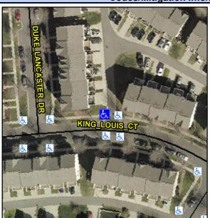
KING LOUIS CT Street 1 Name Stop Condition-Street 2 None Street 2 Name N/A Stop Condition-Street 1 None Possible Solutions: Remove & Replace Curb Ramp With Two New Directional Ramps or Equivalent. Surveyor Notes: N/A PROW/ADA: Not Found, R304.5.1, R304.5.3
