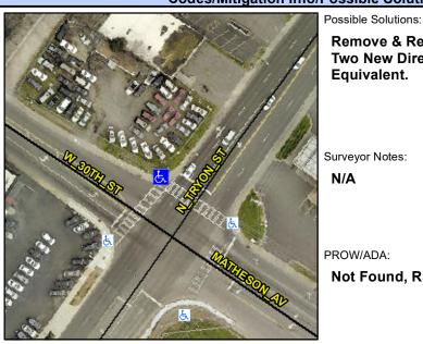
**W 30TH** Street 1 Name Stop Condition-Street 2 Sign Street 2 Name N TRYON Stop Condition-Street 1 Sigr Remove & Replace Curb Ramp With Two New Directional Ramps or Equivalent.
