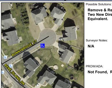
**BONNY BRIDGE CT** Street 1 Name Stop Condition-Street 1 None Street 2 Name N/A Stop Condition-Street 2 N/A Remove & Replace Curb Ramp With **Two New Directional Ramps or** Equivalent.
