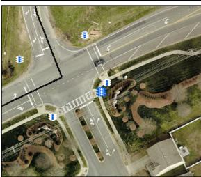
Possible Solutions: Replace Signal Push Button With APS Button on New Post. Remove & Replace Sign.
