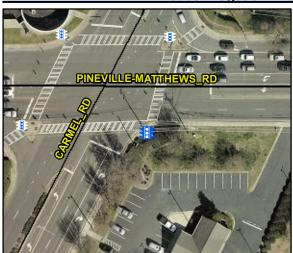
Possible Solutions: Provide Push Button Extension. Remove and Replace Clear Space. Surveyor Notes: N/A PROW/ADA: R404.2, R406.2 1800.00 Total Cost:
