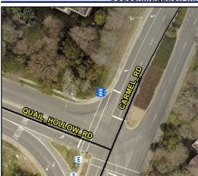
Possible Solutions: Replace Signal Push Button With APS Button on New Post. Remove & Replace Sign.
