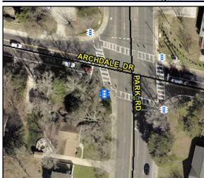
**Compliance Description** Possible Solutions: Provide Push Button Extension. Remove and Replace Clear Space. N/A Signal Buttons Required? Surveyor Notes: N/A PROW/ADA: R404.2, R406.2, R404.3, R404.7.3
