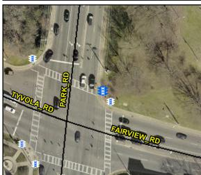
Possible Solutions: Provide Push Button Extension. Remove and Replace Clear Space. Surveyor Notes: N/A PROW/ADA: R404.2, R404.3, R406.2
